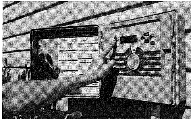
WaterSense-labeled irrigation controllers can significantly reduce overwatering by applying water only when plants need it.
